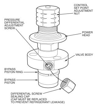
Fig. 13 — Compressor Capacity Control Unloader
